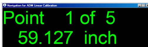
1. Place the target at point 1, which should be roughly three meters from the tracker at any angle. Regardless of the total number of calibration points selected in step 2, the first point should always be taken at 3 meters or greater. Alternately, you can fix a point and move the tracker a similar distance to get the same result. Click on “Pick Up This Point” to continue or “Abort” to cancel without applying any
